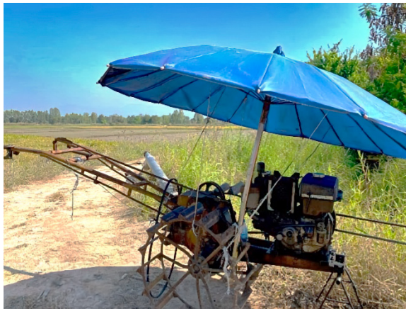
A water pumping machine ( left ), and its connecting pipe made of heavy metal.
