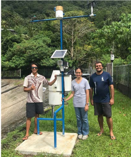
University of Hawai'i researchers worked with staff and interns from the American Sāmoa Power Authority to install weather data collection stations. Stations such as this one collect data that is needed for tracking climate indicators and modeling future change. Photo courtesy of Chris Shuler.
